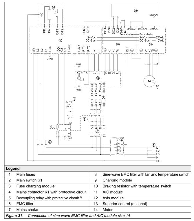
The decoupling relay is not required, if ensured that the load capacitiy of the relais contact is not exceeding, no capacitive load.
