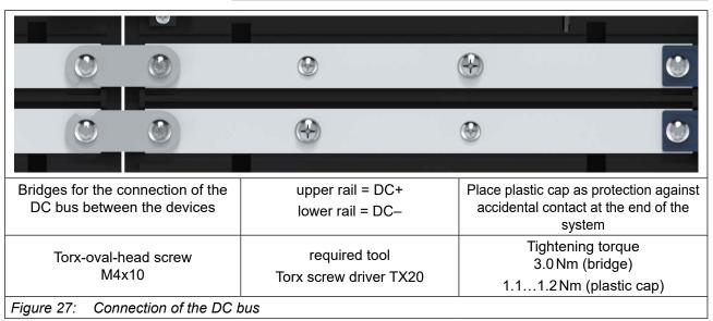
Attach the cover for the DC bus again after the installation.
