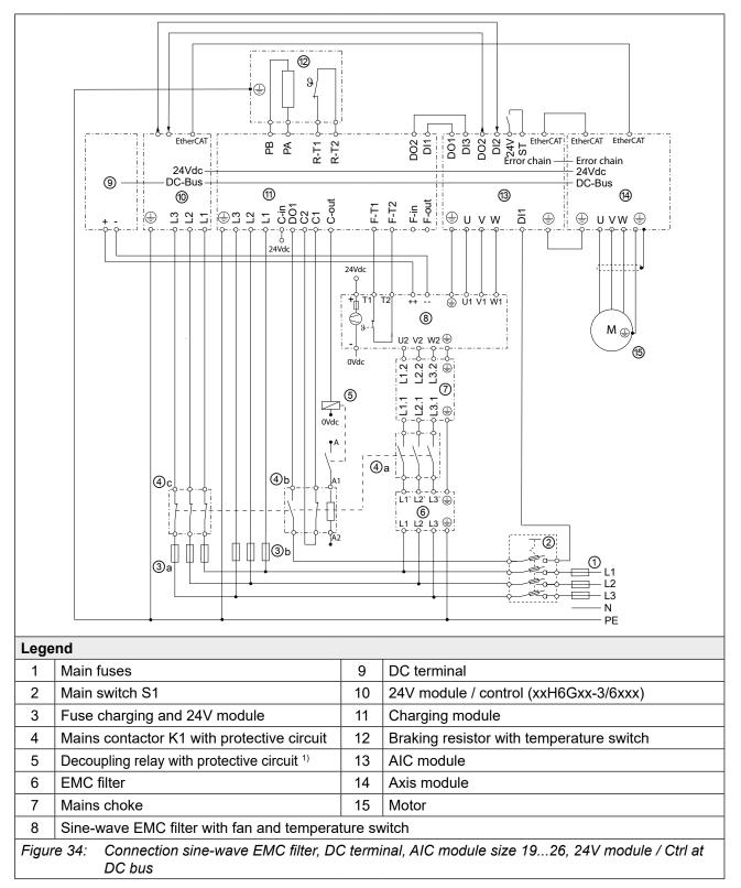
The decoupling relay is not required, if ensured that the load capacitiy of the relais contact is not exceeding, no capacitive load.
