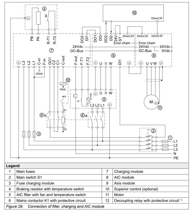
The decoupling relay is not required, if ensured that the load capacitiy of the relais contact is not exceeding, no capacitive load.
