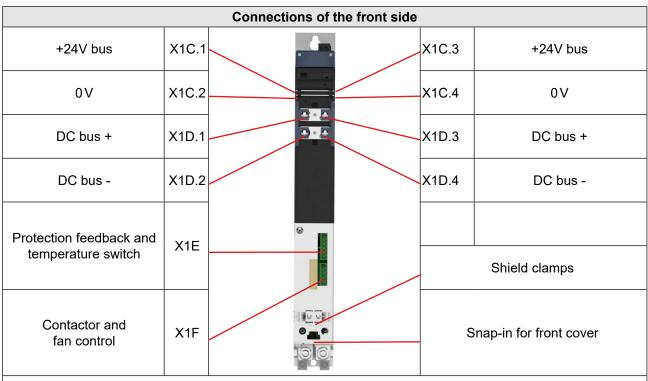
Figure 18: Connections of the front side
