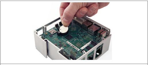
Figure 66: Battery replacement
