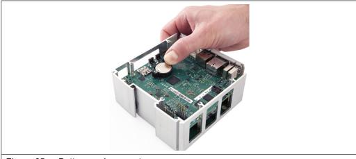
Figure 65: Battery replacement
