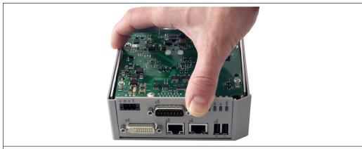
Figure 61: Opening the C6 Smart
