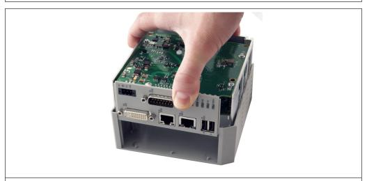
Figure 62: Opening the C6 Smart
