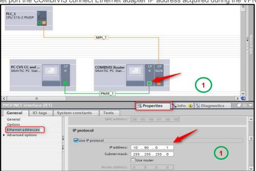
Then perform a click on the green square of the CP IE interface of the COMBIVIS connect router and assign the Ethernet IP address corresponding to the IP address assigned to the LAN ports of the COMBIVIS connect router.
