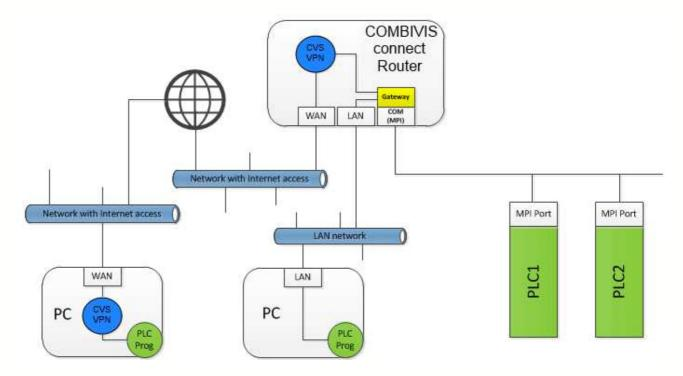
The serial interface of the C6 router (COM) is connected to the MPI subnetwork where several controllers are also connected.
