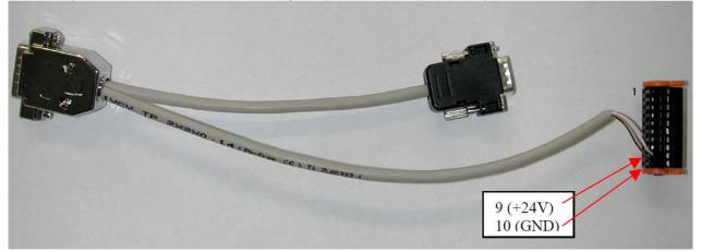
For **P6 and H6** one of the adapter cables must be modified in a way that the 24V (white cable) and GND (brown cable) are connected to the 24V input and GND of the control unit or the control unit must be connected to an external 24V supply.
