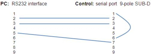
After connecting the cable and before starting the flash procedure the control terminal strip must be provided by 24V (not shown at this picture)!
