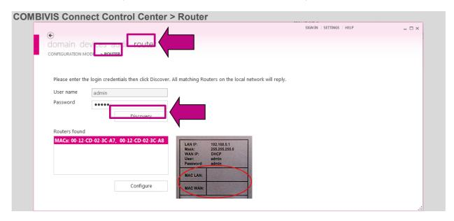
2. Add a static IP-address to the LAN-Port of the router.
