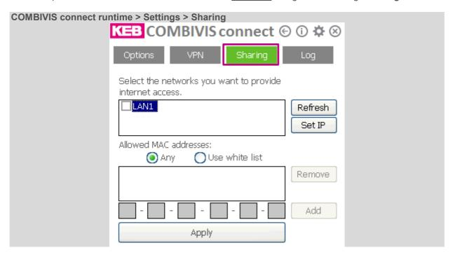
2. Select the Ethernet-adapter, which shall share the internet, and click on "**Set IP**" to insert the needed settings. Set the IP address as static and to the same area as the second network (e.g. production-network). After applying the settings, a reboot of the device is necessary.
