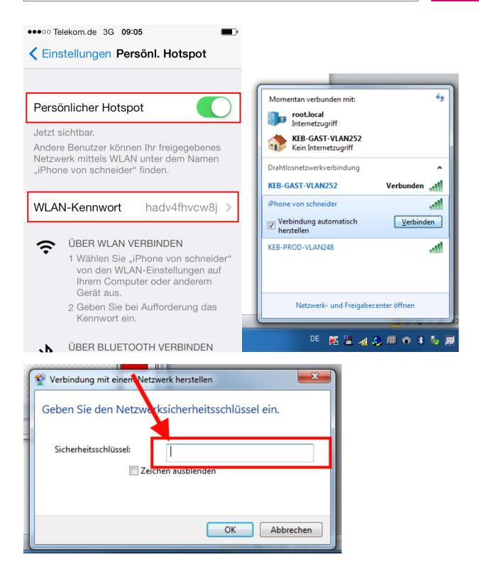
In order to pass through the network connection to the C6HMI or the C6Router, it must be enabled for further participants. At first you open the network and sharing center (*Netzwerk-und Freigabecenter*) after that change the adapter settings (*Adaptereinstellungen ändern*).
