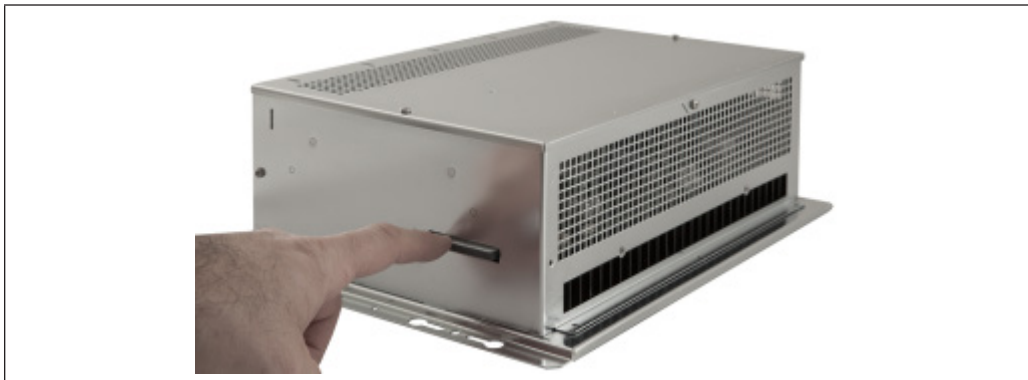
Push and release the memory card as indicated in the figure.
