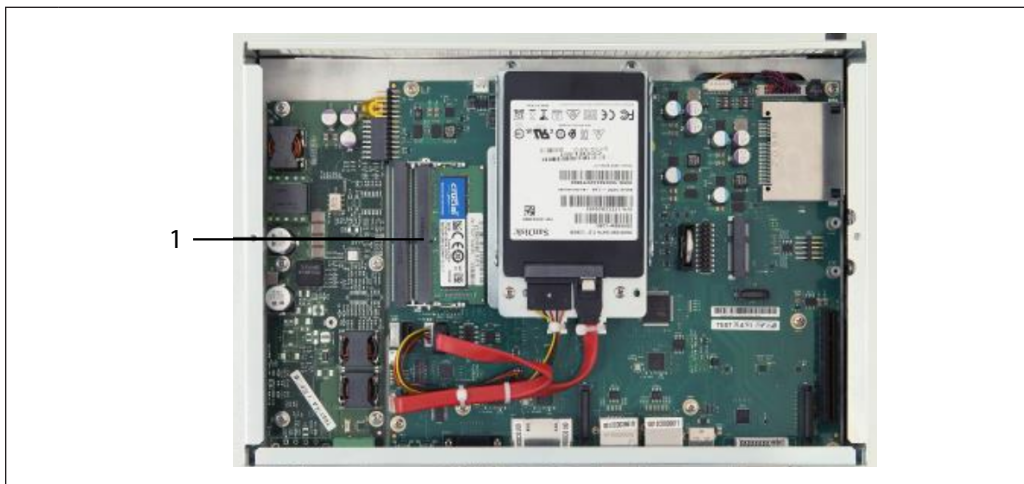
Figure 48: RAM installation / removal
