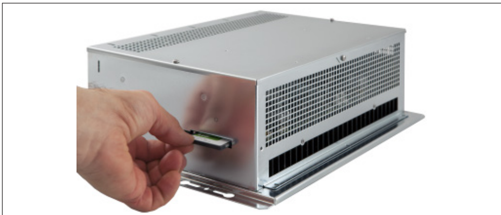
Extract the memory card from the slot.
