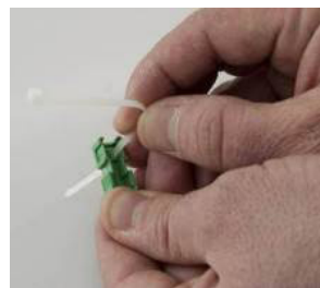
Figure 29: Power connector assembly
