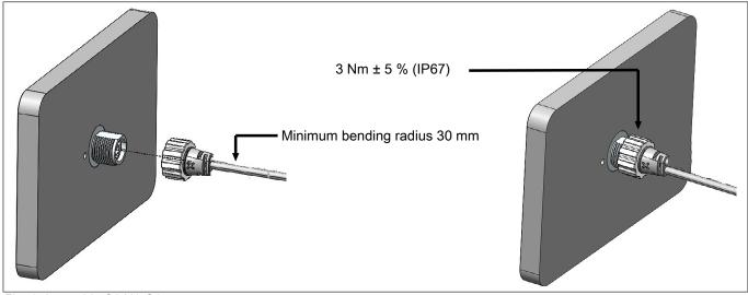
Fig. 1: Assembly C6 X1-C1
