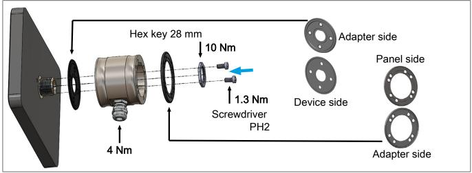
Fig. 1: Assembly C6 X1-M1
