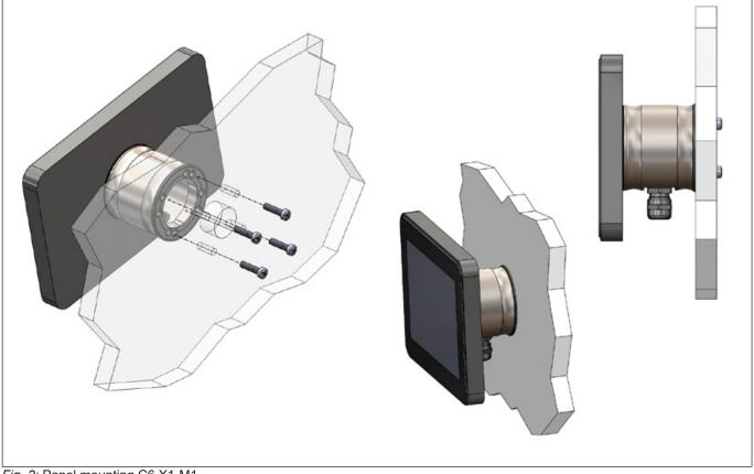
Fig. 2: Panel mounting C6 X1-M1
