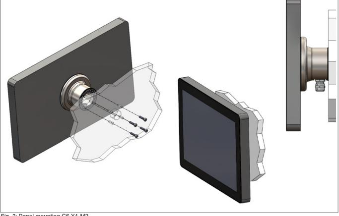
Fig. 2: Panel mounting C6 X1-M2
