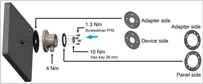
Fig. 1: Assembly C6 X1-M2
