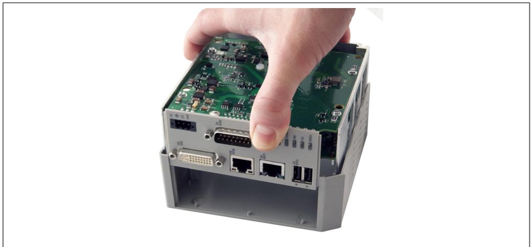
Figure 62: Opening the C6 Smart
