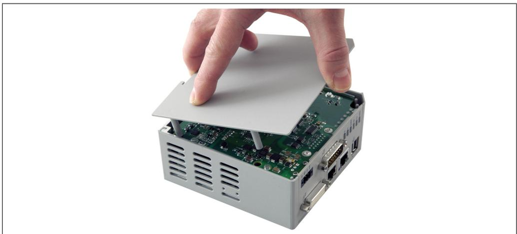
Figure 60: Opening the C6 Smart
