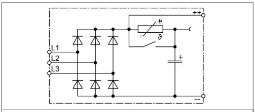
Figure 12: Input wiring / drive controller type
