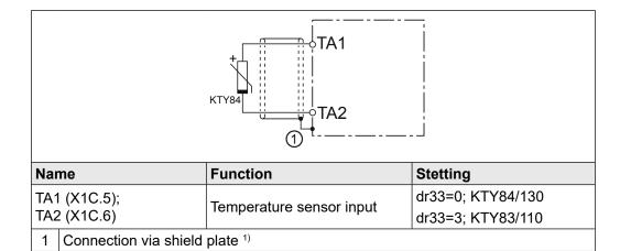
Figure 24: Connection of a KTY sensor for K- and A-control
