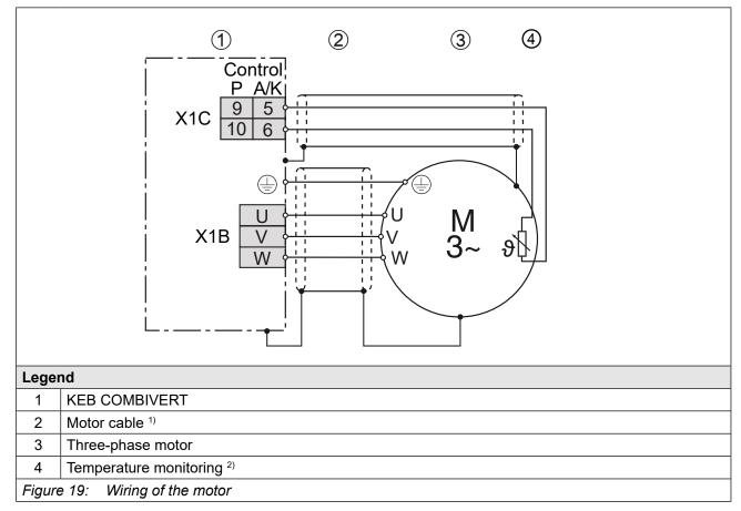
Apply the shield at both ends over a large area on the functional earth (shielding plate or mounting plate)
