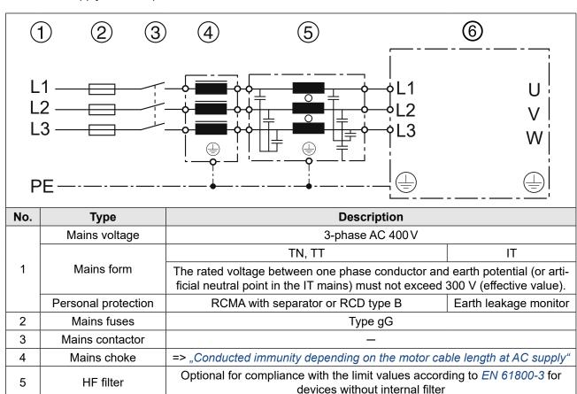
Figure 15: Connection of the mains supply
