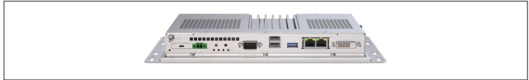
C6 E22 BOX/PANEL "SL" (slim form) has no PCI/PCIe slot.
