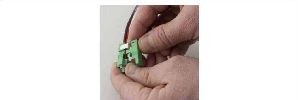
Figure 58: Power connector installation
