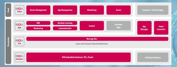
The core infrastructure on the edge component (NOA Core) is based on a Linux and container-based architecture and can be used on embedded hardware, IPCs and panels from KEB or 3rd party devices. The App Manager is used to operate NOA apps such as solutions for HMIs, machine learning (anomaly detection and predictive maintenance), monitoring and control systems as well as customised or 3rd party apps.
