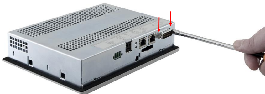
Figure 73 Backup battery replacement
