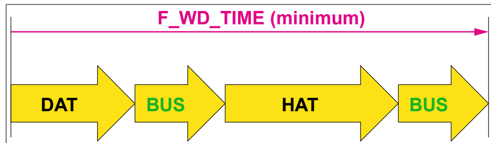
Fig. 3: Response time safety module type 3 with PROFIsafe
