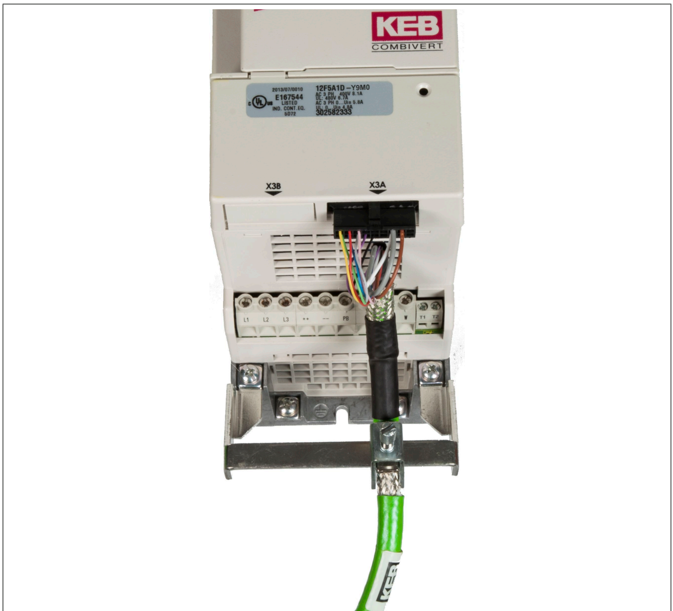
Figure 4: encoder cable shield with shielding clamp on grounding bar“).
