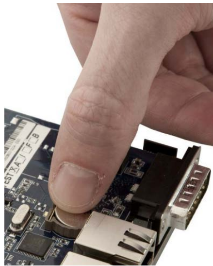
Figure 52: Backup battery replacement
