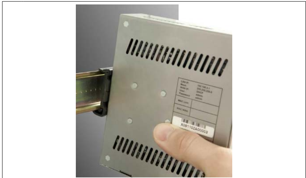
Figure 25: Wall mounting procedure / DIN rail mounting
