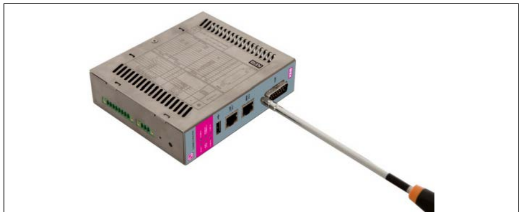
Figure 48: Backup battery replacement
