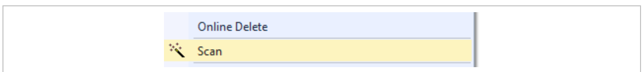
Figure 4: TwinCAT: Scan for Ethercat devices
