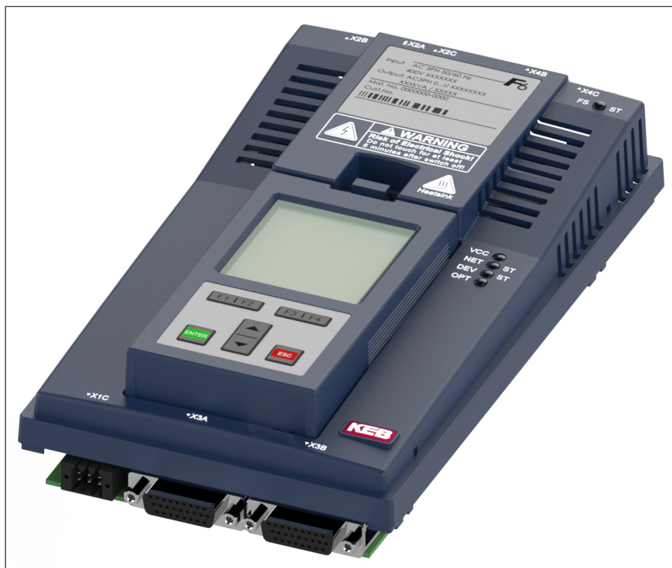
Fig. 2: Control card block incl. operator (front panel)
