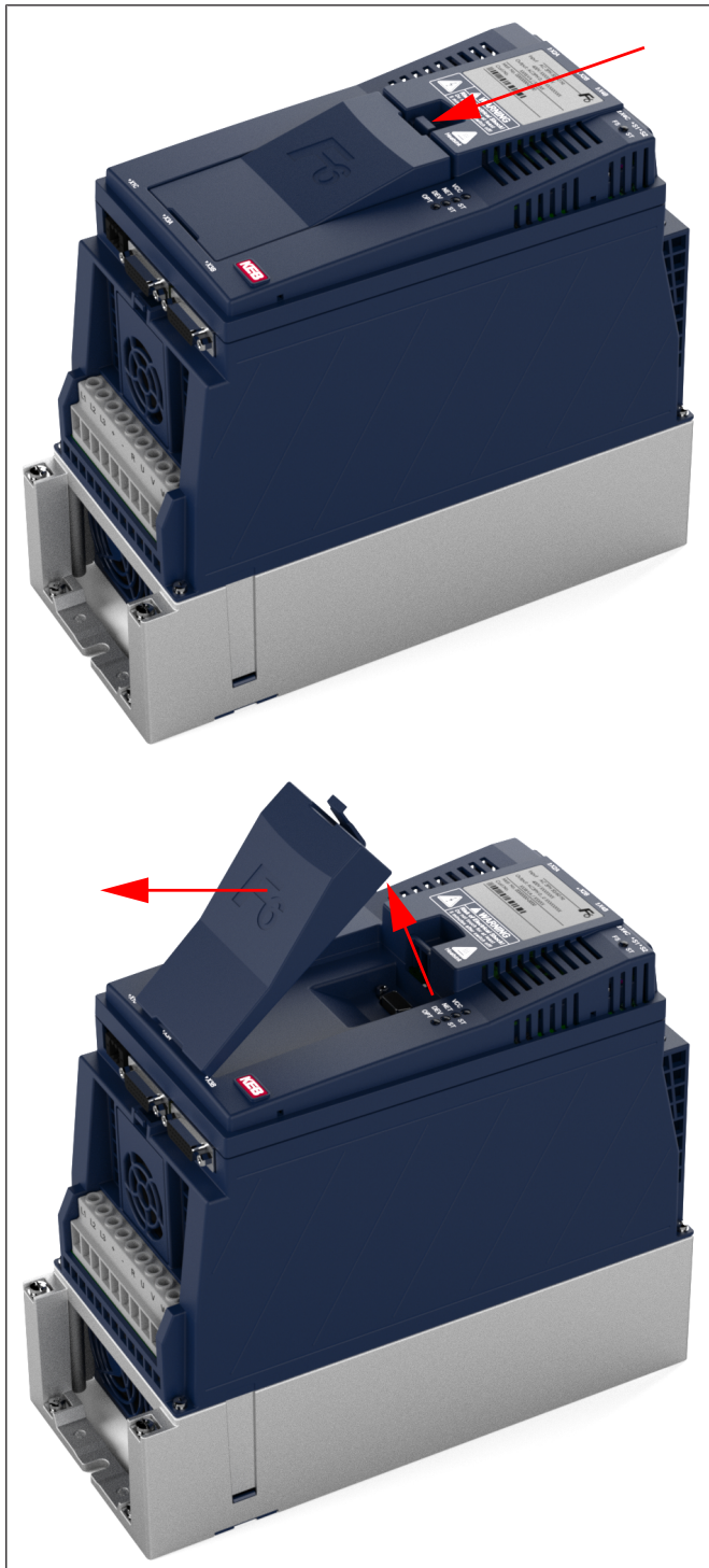
Fig. 6: Remove the blind cover
