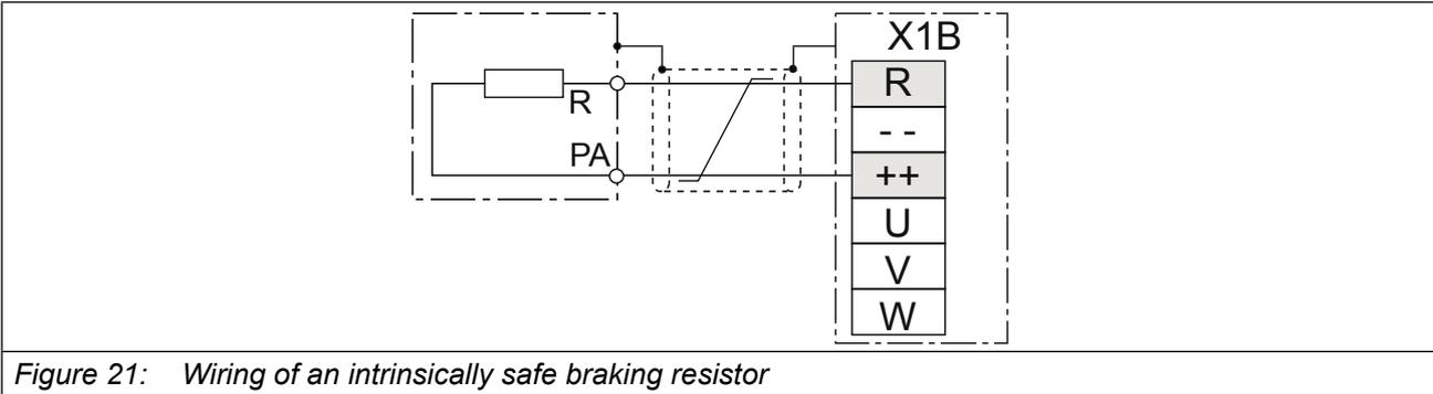
Figure 21: Wiring of an intrinsically safe braking resistor
