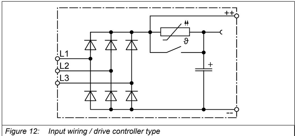
Figure 12: Input wiring / drive controller type
