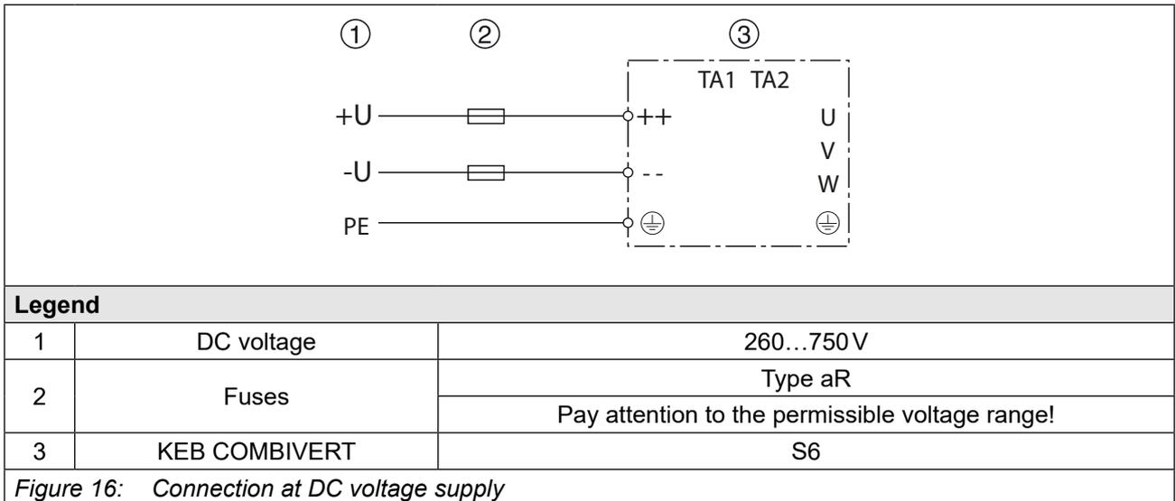
Figure 16: Connection at DC voltage supply
