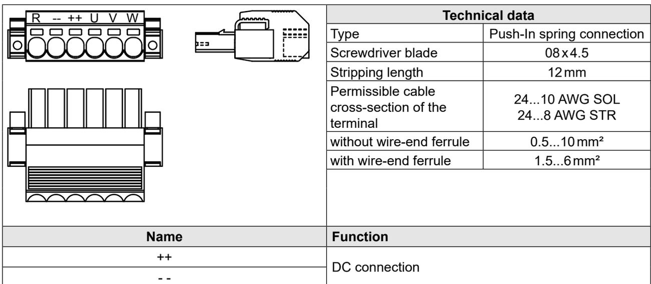
Figure 17: Terminal block X1B DC connection
