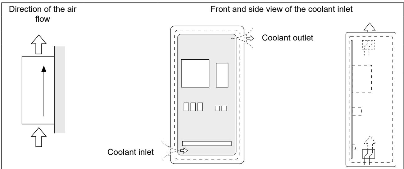
Figure 4: Control cabinet ventilation
