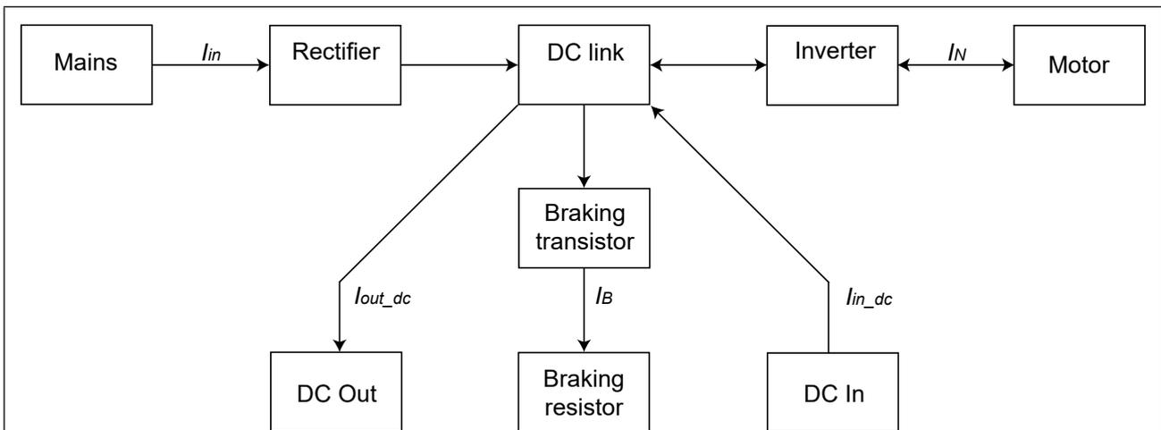
Figure 9: Block diagram of the energy flow
