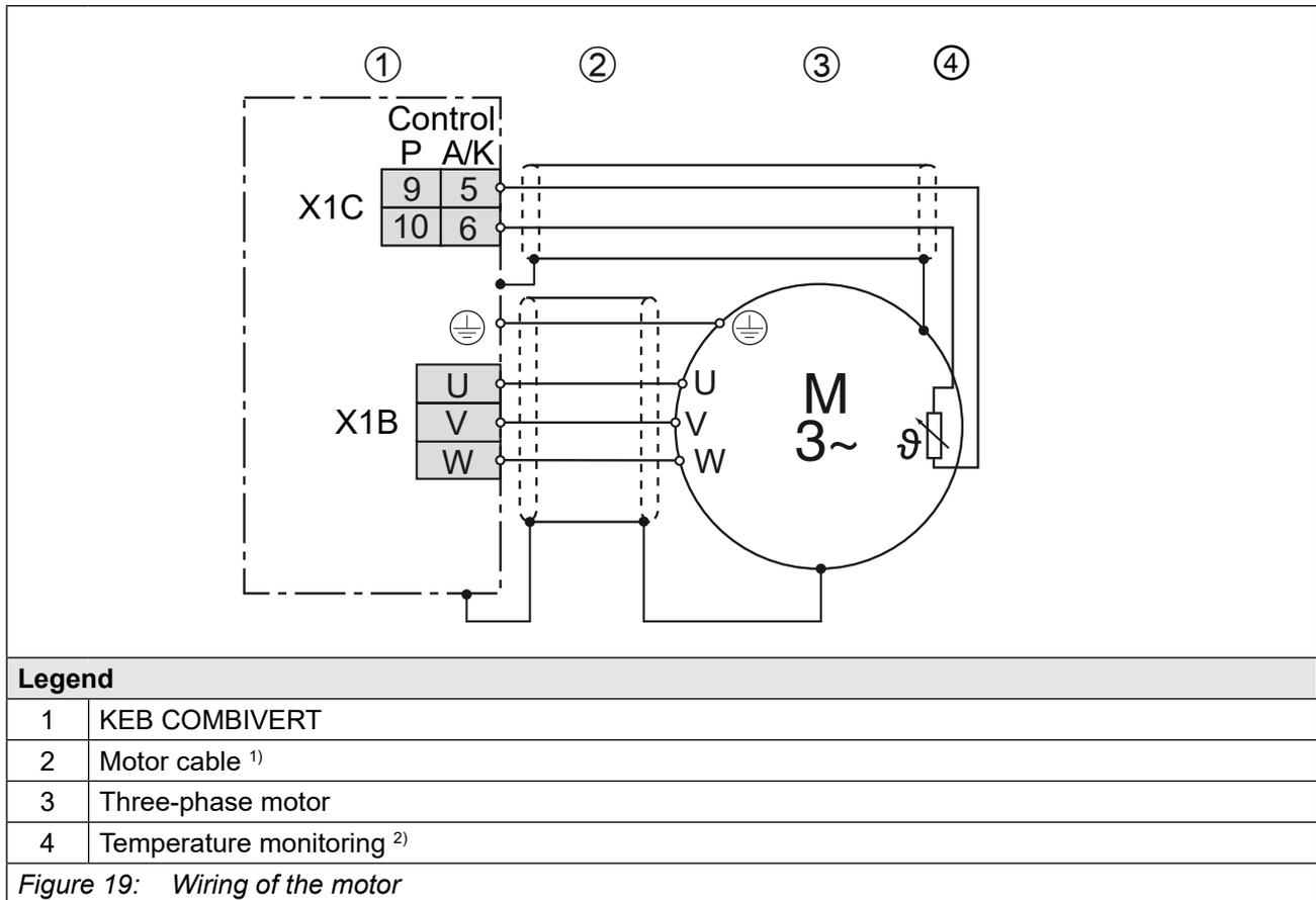
Figure 19: Wiring of the motor
