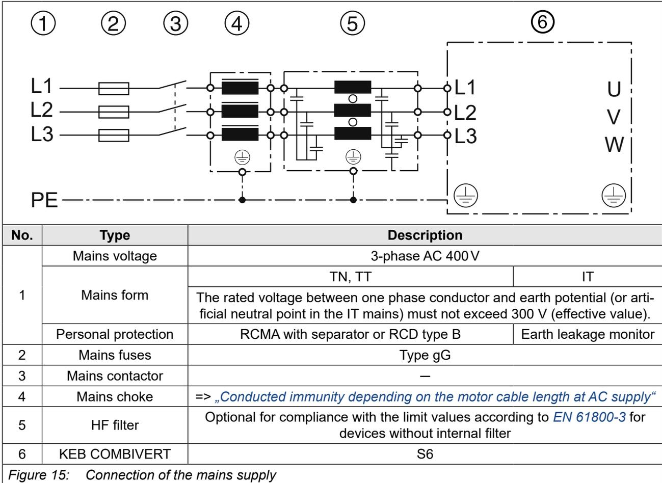
Figure 15: Connection of the mains supply
