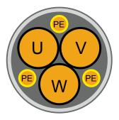
It is recommended to use symmetric shielded motor cables at high motor ratings (>30 kW). At these cables the protective earth conductor is tripartited and uniformly placed between the phase lines.
