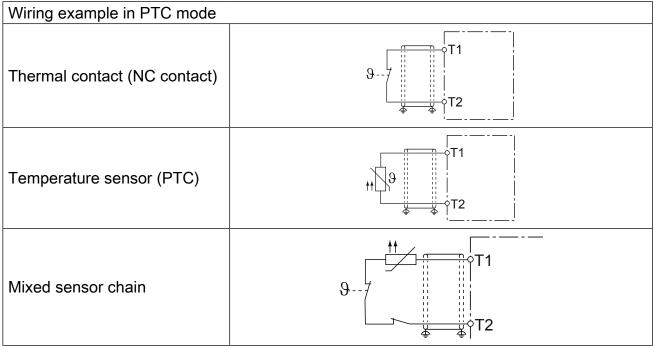
The function can be switched off with Pn.12="7" (CP.28) if no evaluation of the input is desired (standard in operating mode GENERAL). Alternatively a bridge can be installed between T1 and T2.
