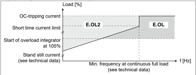
A PT1 element ( $\tau$  = 280 ms) starts if the permissible current is exceeded. After its sequence of operation the error E.OL2 is triggered.
