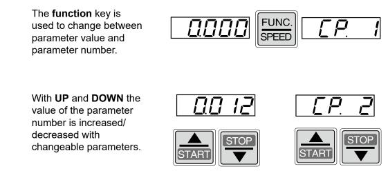
Principally during a change, parameter values are immediately accepted and stored non-volatile. However, with some parameters it is not useful that the adjusted value is accepted immediately. When this type of parameter is changed a point appears behind the last digit.
