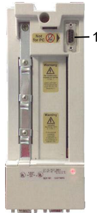
Fig. 14: Connection of COMBIVERT F5 terminal X4A
