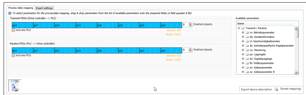
Fig. 226: Wizard - Fieldbus - Create Powerlink xdd
