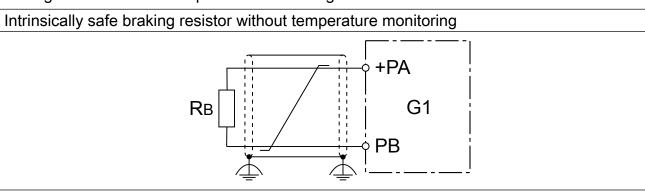
Figure 13: Braking resistor without temperature monitoring
