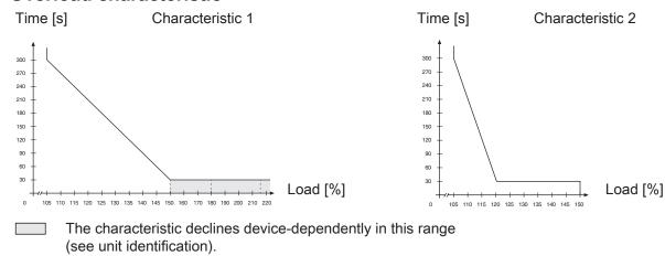
On exceeding a load of 105% the overload integrator starts. When falling below the integrator counts backwards. If the integrator achieves the overload characteristic that corresponds to the inverter, the error E.OL is triggered.
