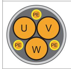
It is recommended to use symmetric shielded motor cables at high motor ratings (>30 kW). At these cables the protective earth conductor is tripartited and uniformly placed between the phase lines.
