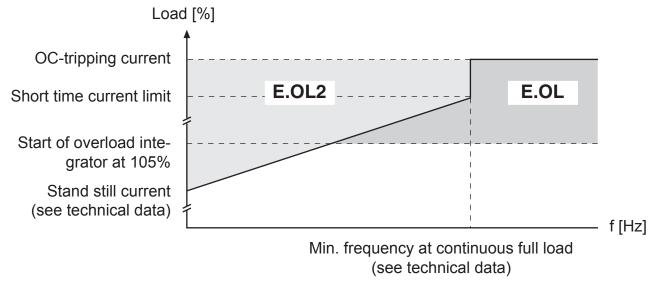
A PT1-element ( $\tau$  = 280 ms) starts if the permissible current is exceeded. After its sequence of operation the error E.OL2 is triggered.
