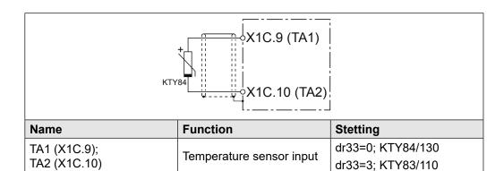
Figure 29: Connection of a KTY sensor for P-control
