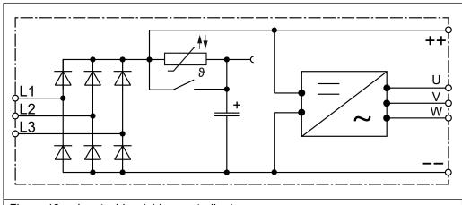
Figure 13: Input wiring / drive controller type
