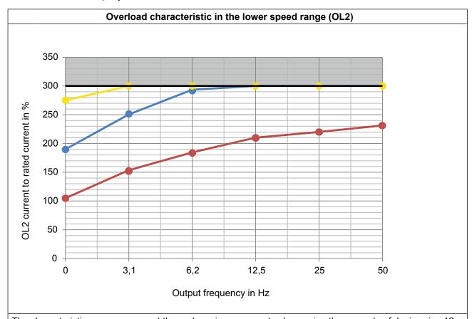
The characteristic curves represent the real maximum current values using the example of device size 12.
