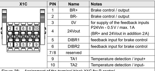
Figure 28: Assignment of the terminal block X1C for P-control
