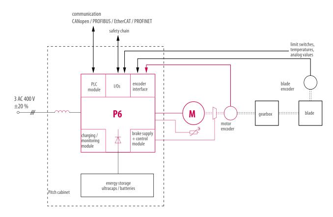
By using the highly integrated KEB P6, just very few components are needed externally in the cabinet.
