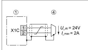
The voltage to the control of a brake is decoupled from the internal voltage supply. The brake works only with external voltage supply.
