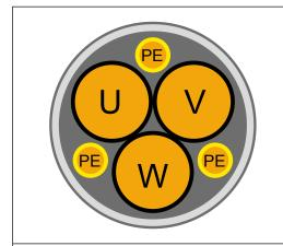
The use of shielded motor lines with symmetrical structure is required for higher motor power (from 30 kW). In these lines the protective earth conductor is tripartite and evenly arranged between the phase lines. A cable without protective earth conductor can be used if local regulations so permit. Then the protective earth conductor must be laid externally. Certain lines also permit the shield for the use as protective earth conductor. For this, observe the details of the line manufacturer!
