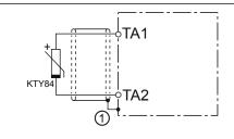
KTY sensors are polarized semiconductors and must be operated in forward direction!
