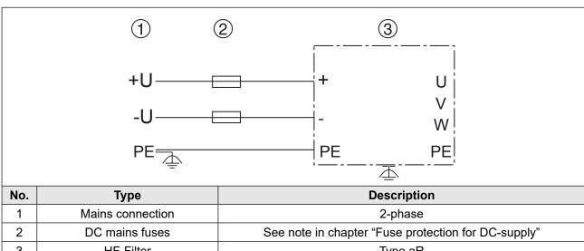
2 DC mains fuses See note in chapter "Fuse protection for DC-supply"
