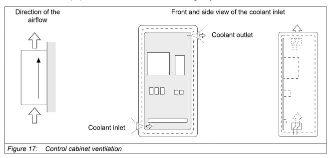
4.2.7 Airflow of the drive converter
