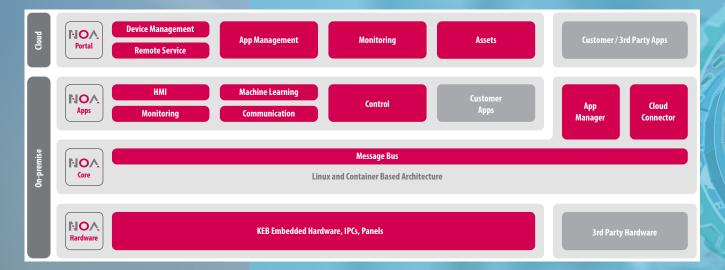
The core infrastructure on the edge component (NOA Core) is based on a Linux and container-based architecture and can be used on embedded hardware, IPCs and panels from KEB or 3rd party devices. The App Manager is used to operate NOA apps such as solutions for HMIs, machine learning (anomaly detection and predictive maintenance), monitoring and control systems as well as customised or 3rd party apps.
