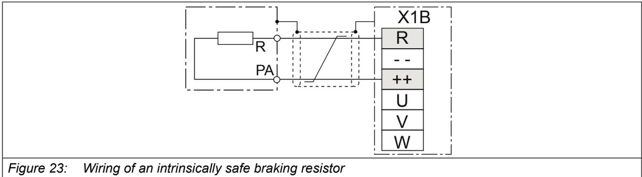
Figure 23: Wiring of an intrinsically safe braking resistor
