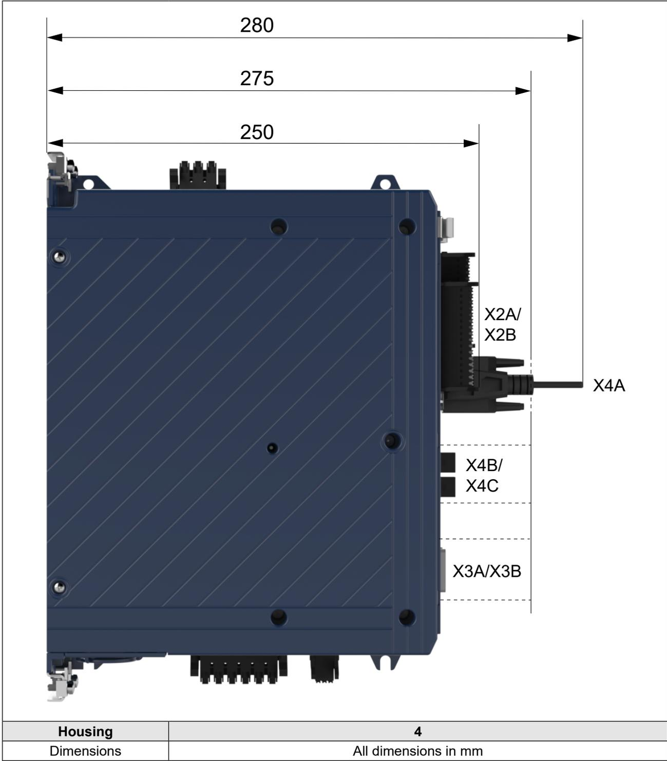
Figure 6: Installation depth
