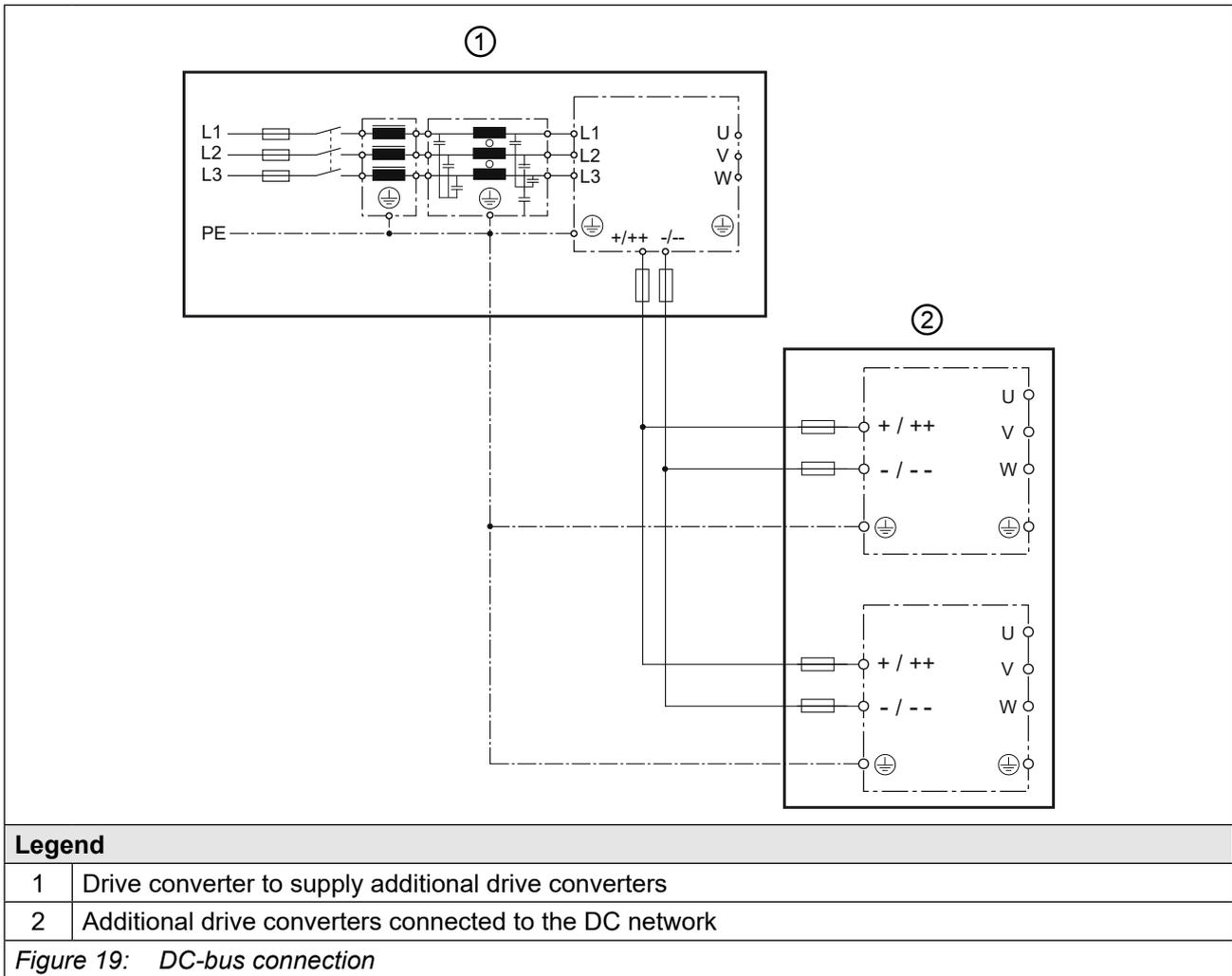
**① When using this drive converter to supply additional drive converters via the DC terminals, the following must also be observed:**
