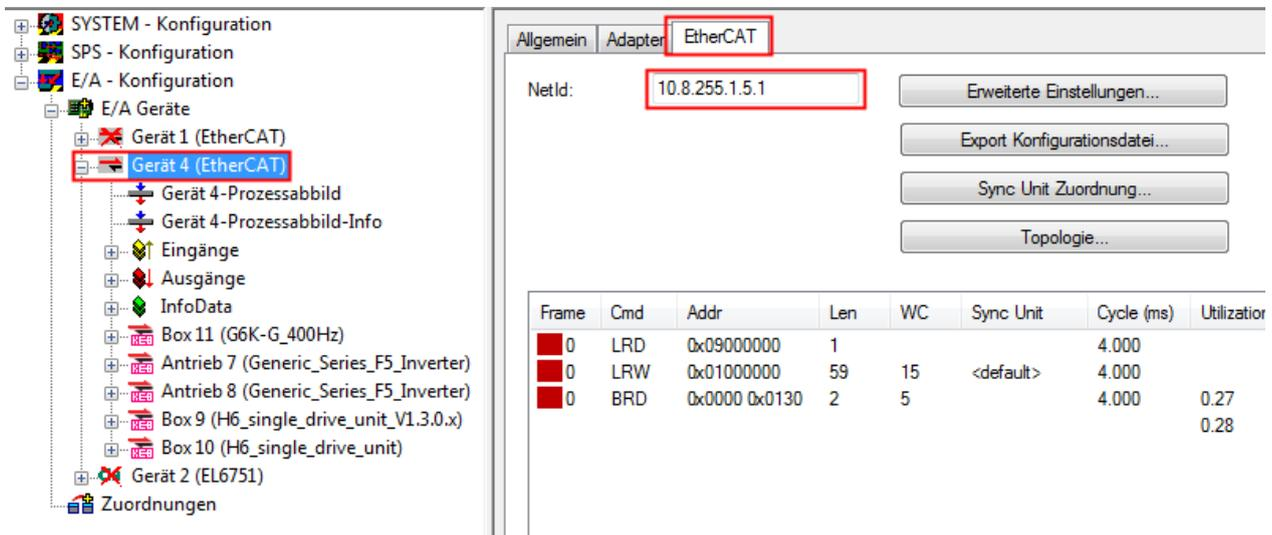
The screenshot shows the 'EtherCAT' configuration window for 'Gerät 4'. The 'NetId' field is set to '10.8.255.1.5.1'. Below the configuration fields is a table showing the EtherCAT configuration for the device.
