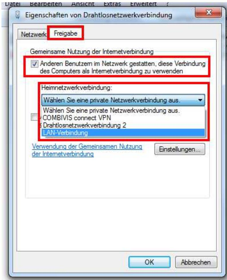
Now the network port of the C6 HMI / C6 Router is to be determined under the menu tab „Sharing“ (*Freigabe*). Select the network port which is connected to your laptop.
