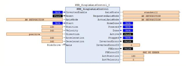
Now you can see the position currently set on the module at ActPosition. Now the module must be changed to the AxisMode (required for operation) again.
