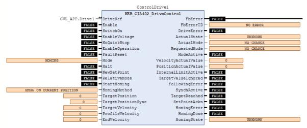
Subsequently the module must be connected with the *DriveRef* and can be started via the input *Enable*. The *HomingMethod* must be set to value 35 (HM35 On Current Position). Now if you set the input *StartHoming* to True, the value written onto parameter *Home offset* is written to *position actual value*. The successful homing is represented with the output *HomingDone*.
