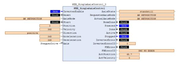
The value which shall be entered now in Position actual value must be entered in Position. Then start the module with Start, a feedback is given via the Variable Done.
