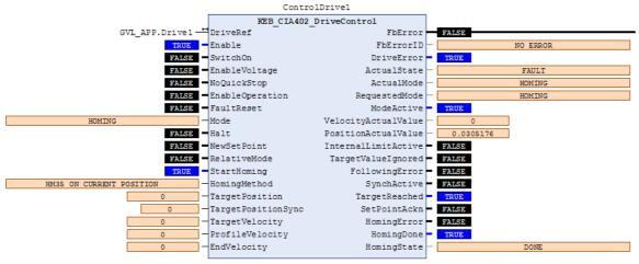
Now you can see the transferred value in the EtherCAT E/A image of the module under parameter Position actual value.
