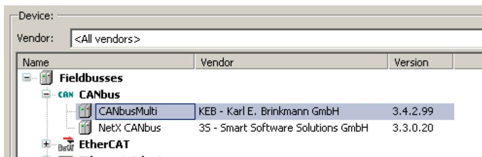
Now we need to add a CANopen\_Manager object to the CANbusMulti device. You can simply do that with left clicking on the recently added CANbus device if the add device dialog is still open.
