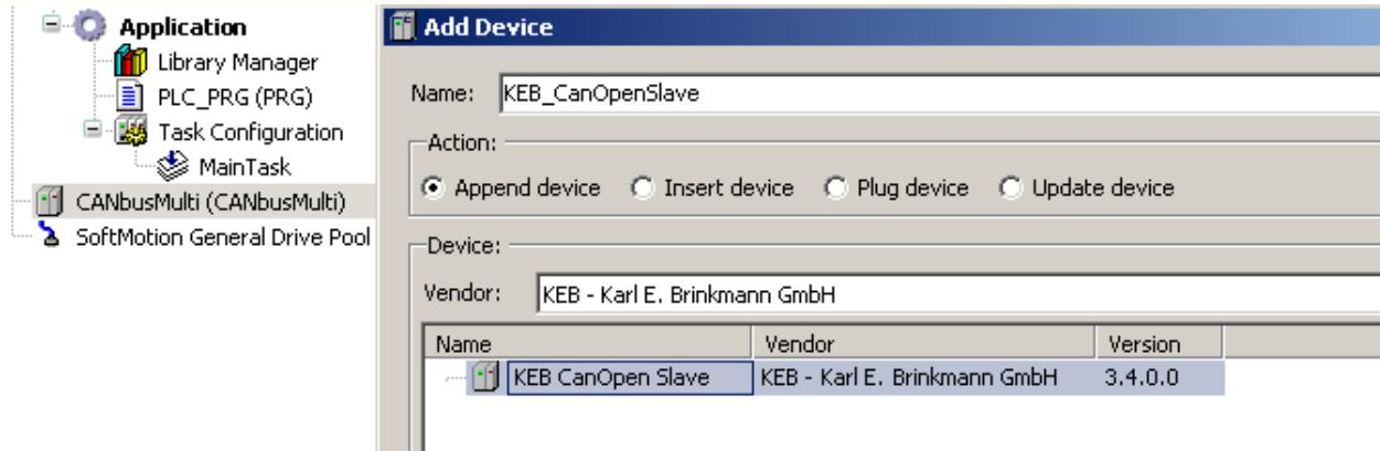
Now the difficult part: setting up the ObjectDictionary. It is highly recommended to use the CANopenDevice sample project which is installed with Combinis studio 6 but you can find the needed source code in the appendix.
