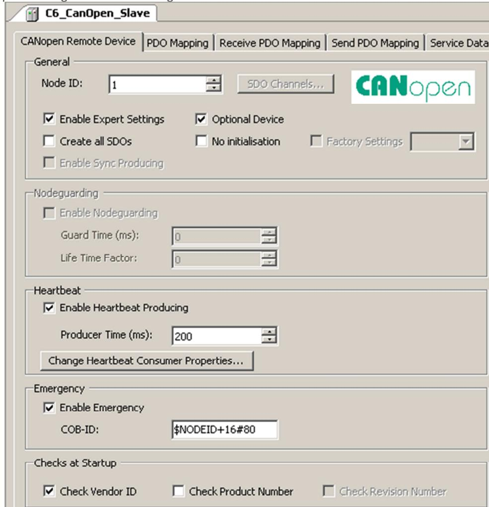
You have two possibilities for bus monitoring. One method is the heartbeat producing (must be enabled in master and slave with identic producer time). The second method is the so called Nodeguarding. To enable the checkboxes for Nodeguarding you must uncheck "Enable Heartbeat Producing" and disable the consumer properties.
