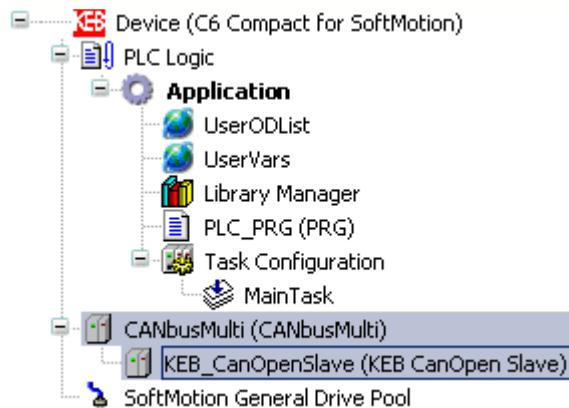
The process data is mapped to the User Object Dictionary. You can use the Arrays for your PDO data.
