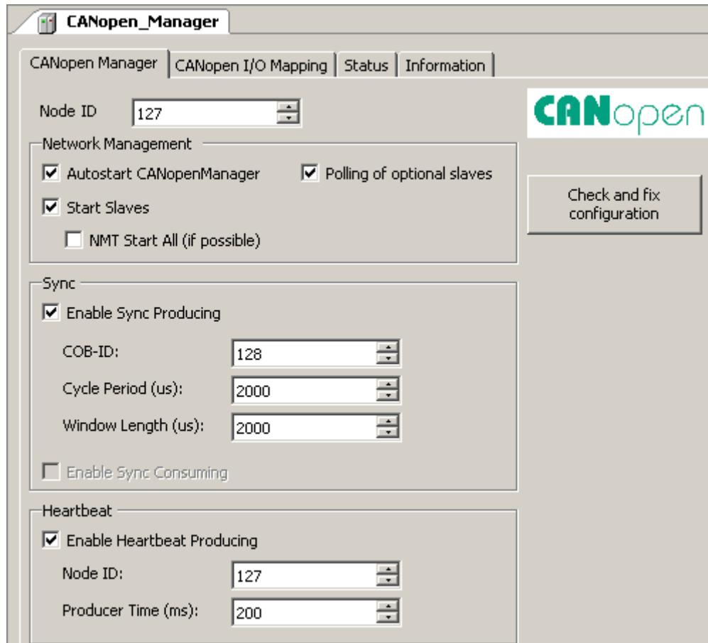
The CANopen\_Manager is the Master device and controls some basic CAN features.
