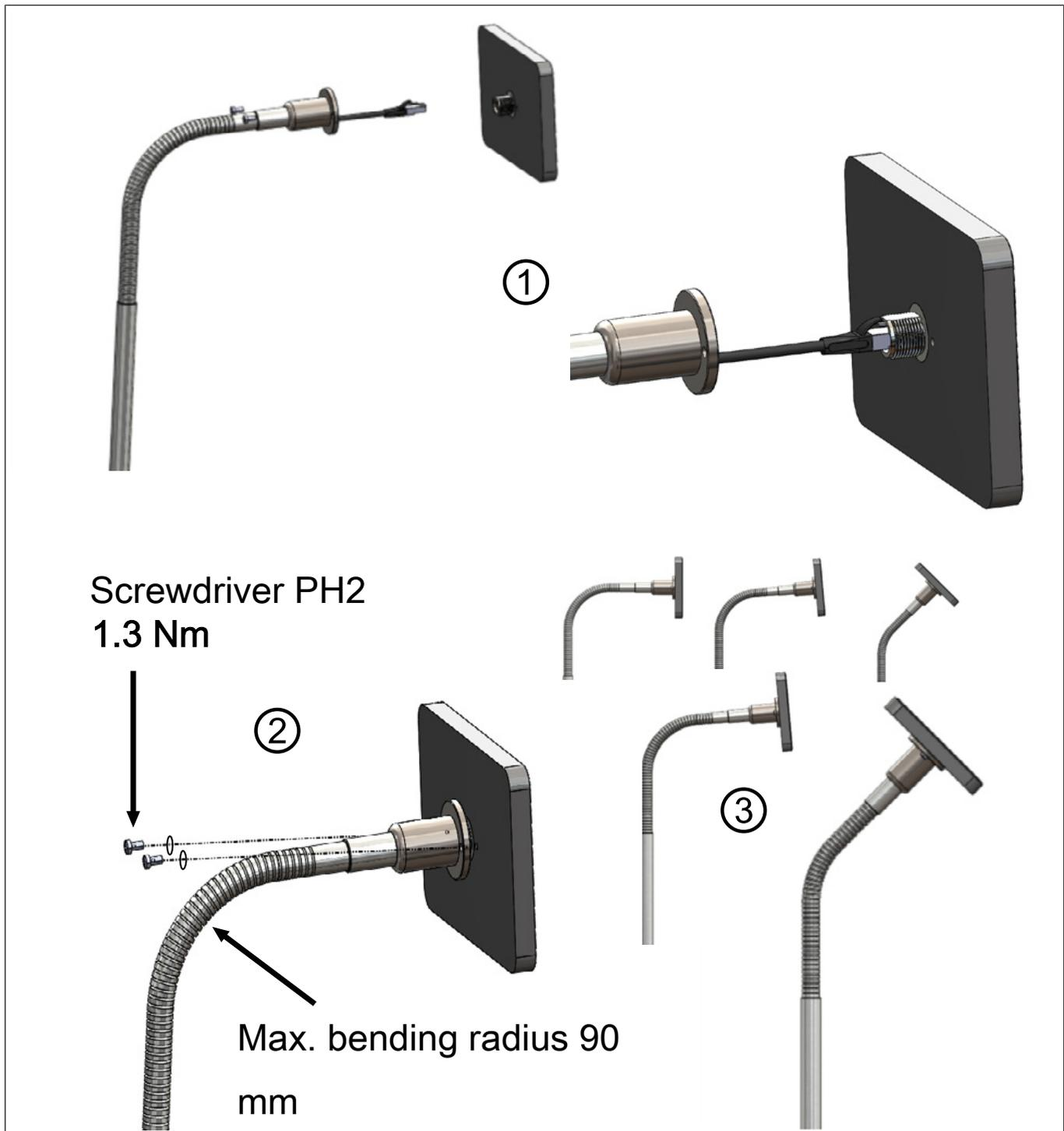
Fig. 2: Monitor assembly C6 X1-G1
