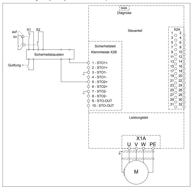
With operation of the emergency stop unit, e.g. by protection door, the release paths of the safety module are disconnected. This leads to the loss of the STO signals (X2B.1 and 5) and thus to energy disconnection of the drive. The safety module makes a consistency check of all signal paths via test signals (OSSD).
