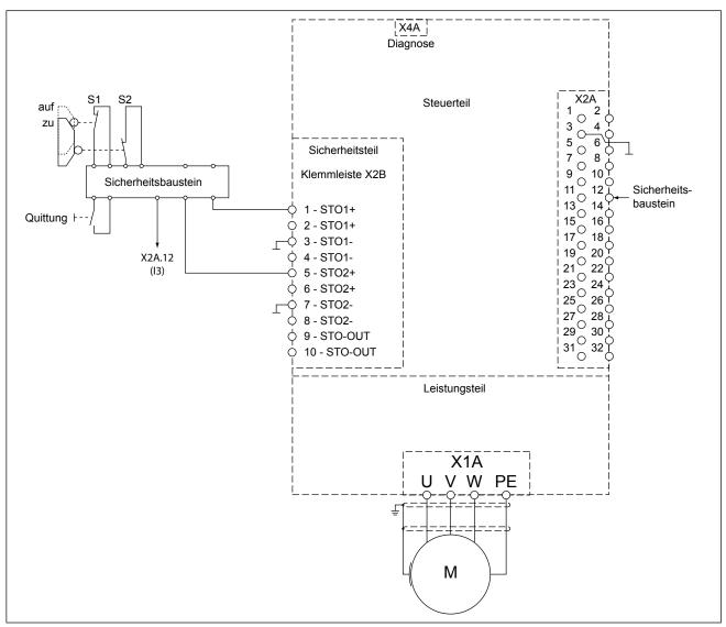
By activation of the emergency stop unit the drive is stopped with a deceleration ramp via input X2A.12 (I3).
