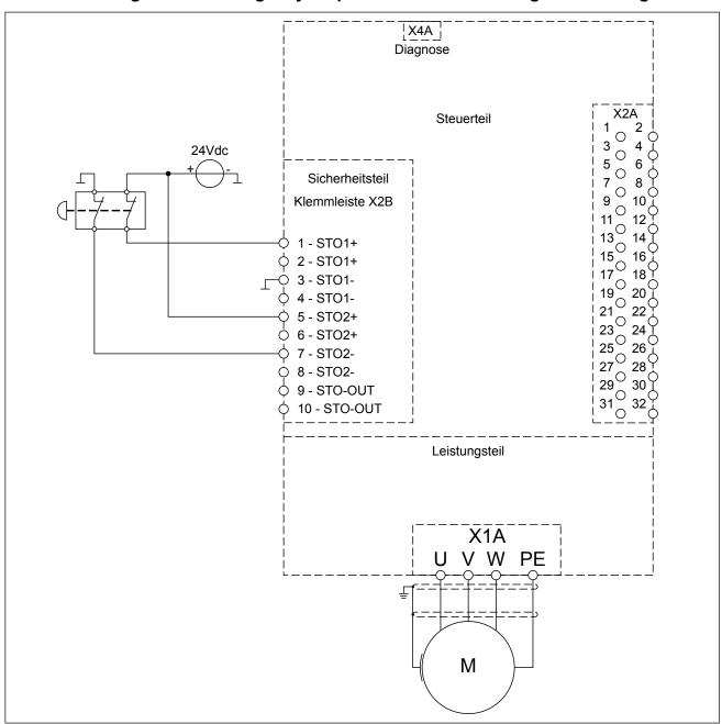
The displayed circuit shows wiring errors in the area of the emergency stop unit and supply line. A possible short circuit on the primary side of the emergency stop switchgear (mass and 24 Vdc) and a short circuit on the secondary side of the unit or within the wiring leads either directly or with closed contacts to a short circuit of the supply, whereby a series-connected 24V fuse triggers.
