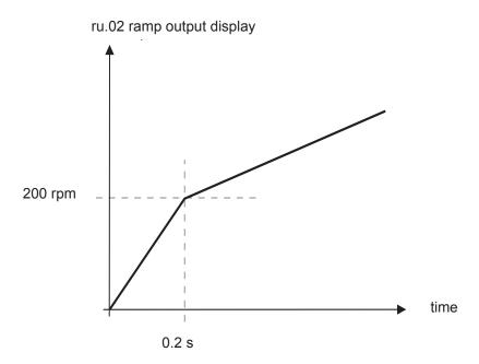
ud.02 "control type" = 4 (4000 rpm mode) dS.21 "ASCL startup speed" = 200 rpm dS.22 "ASCL startup time" = 1s
