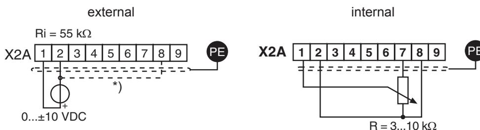
Analog set value setting in torque regulated operation (CP.10 = 5) and reference source CP.28 = 1:
