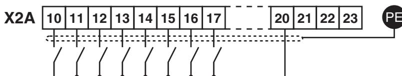
Using of an external voltage supply
