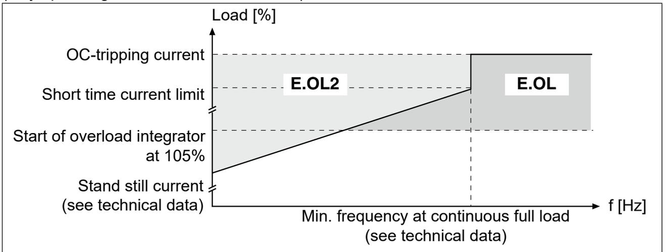
A PT1 element ( $\tau = 280 \text{ ms}$ ) starts if the permissible current is exceeded. After its sequence of operation the error E.OL2 is triggered.
