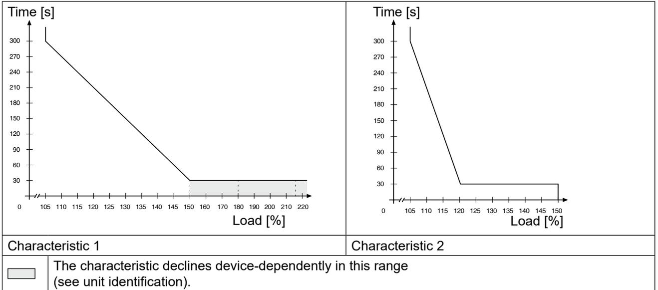
On exceeding a load of 105% the overload integrator starts. When falling below the integrator counts backwards. If the integrator achieves the overload characteristic that corresponds to the inverter, the error E.OL is triggered.
