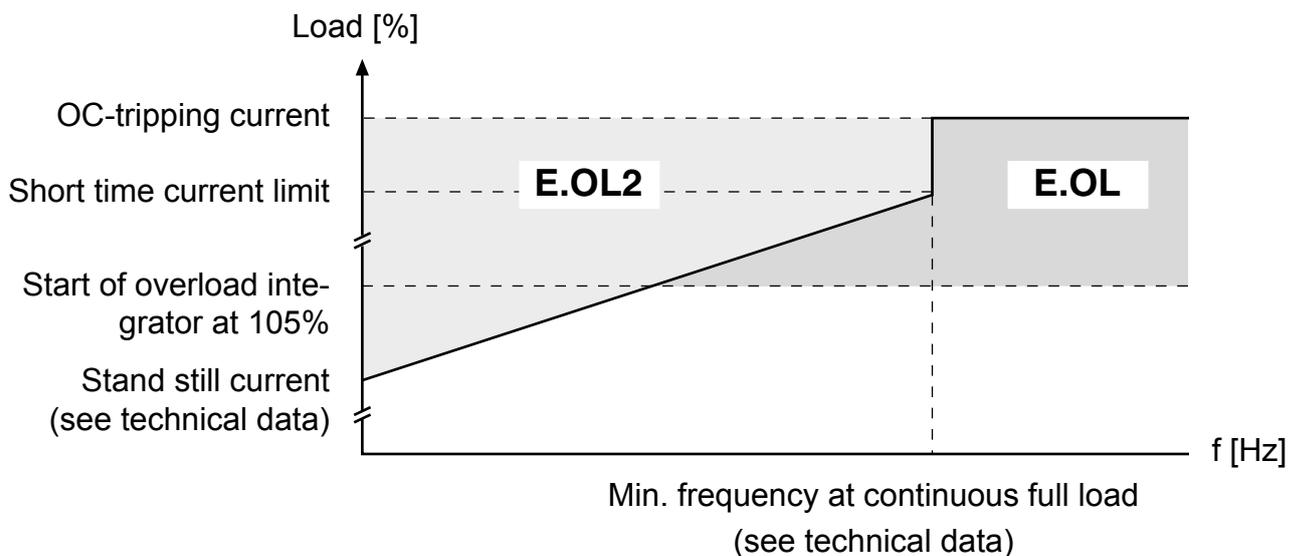
Figure 15: Overload protection in the lower speed range
