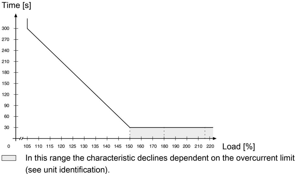
Figure 14: Overload characteristic
