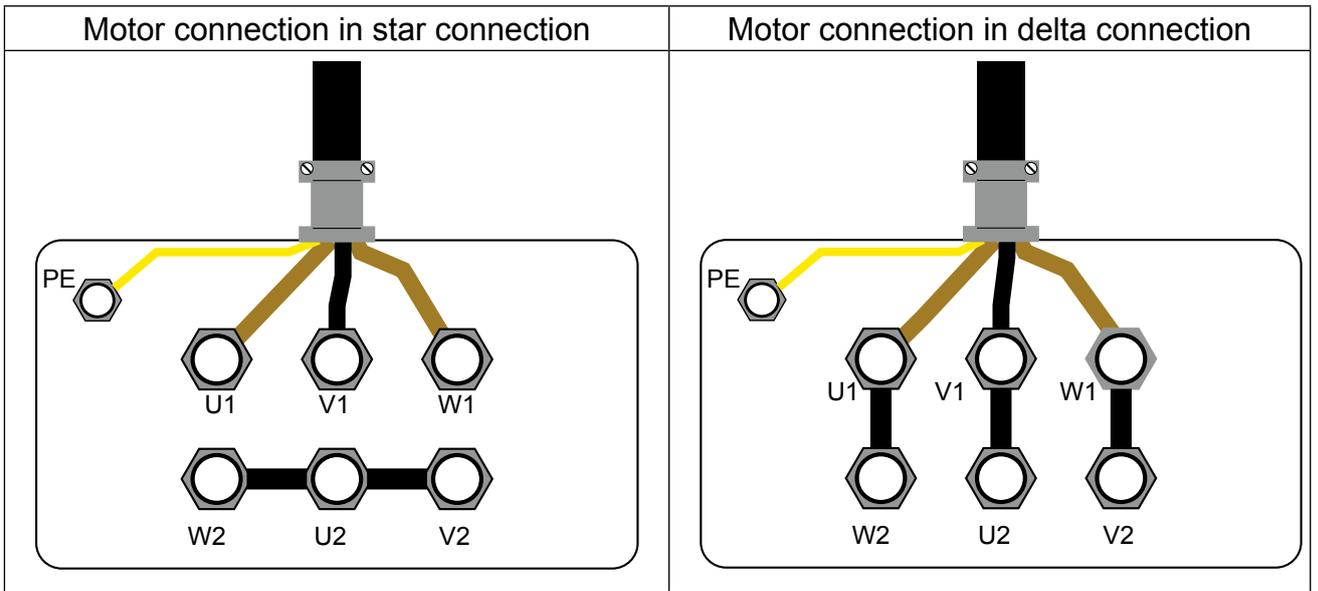
Figure 10: Connection of the motor
