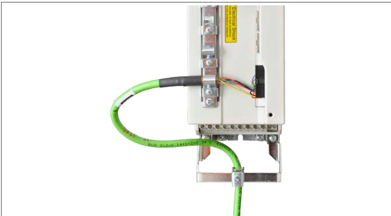
Strain relief at housing D by use of mounting kit B0F5T88-0001 or -0002
