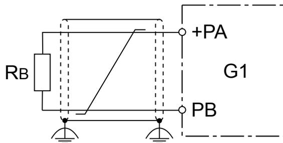
Figure 12: Braking resistor without temperature monitoring
