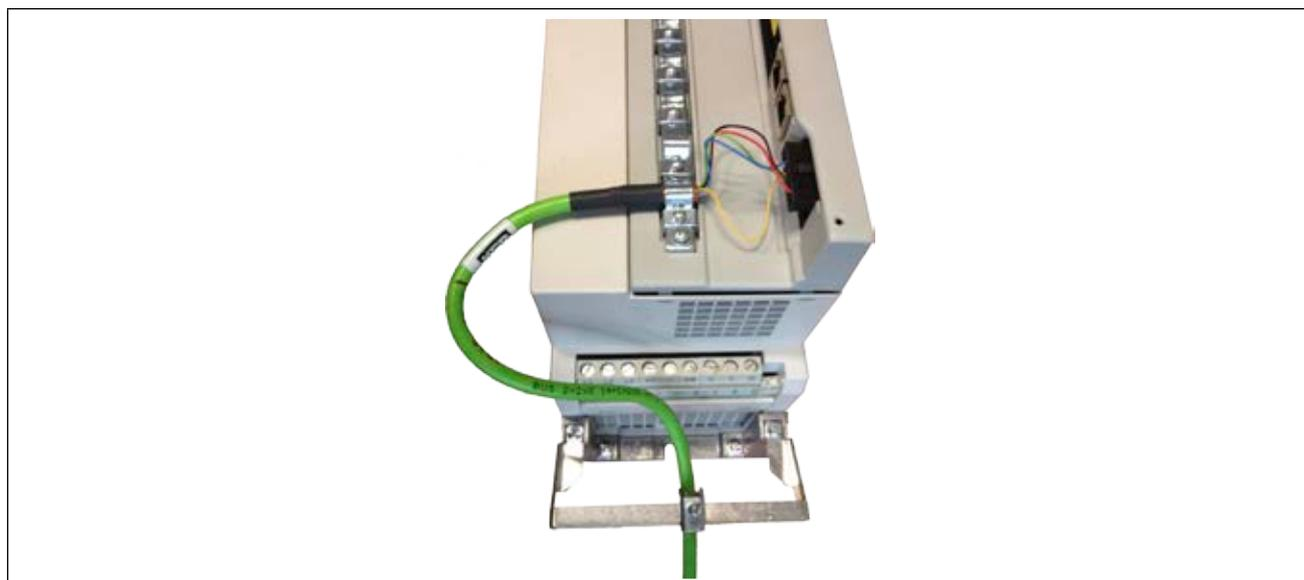
Strain relief at housing E by use of mounting kit E0F5T88-0001 or -0002
