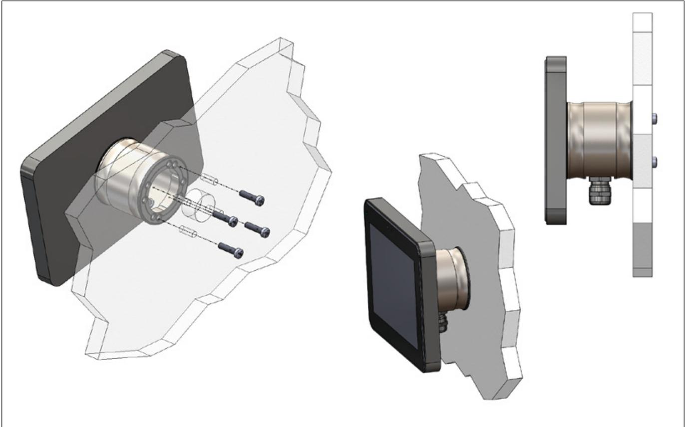
Fig. 2: Panel mounting C6 X1-M1
