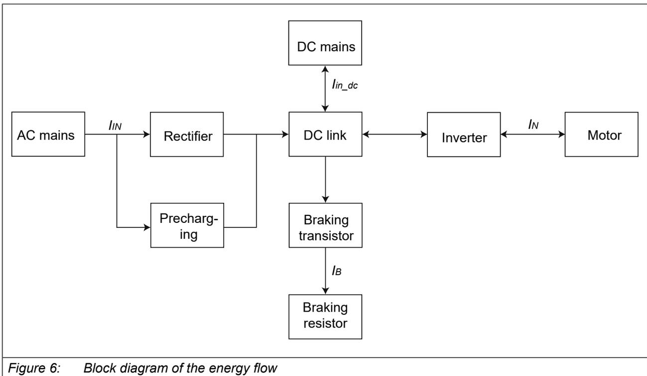
Figure 6: Block diagram of the energy flow
