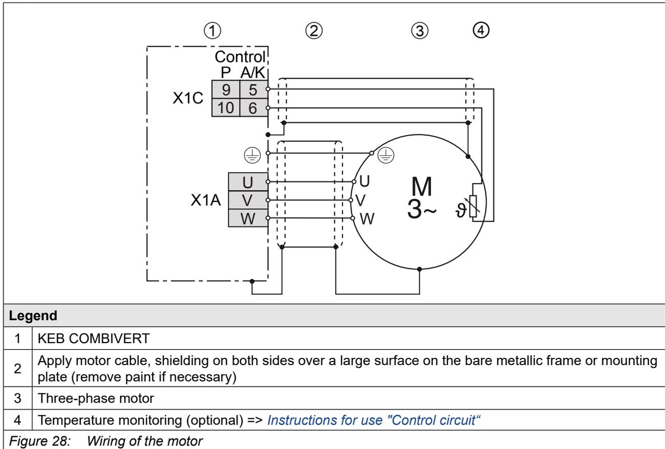
Figure 28: Wiring of the motor
