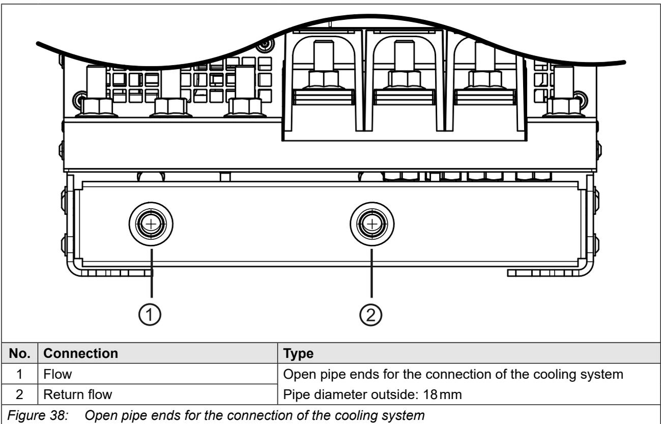
Figure 38: Open pipe ends for the connection of the cooling system
