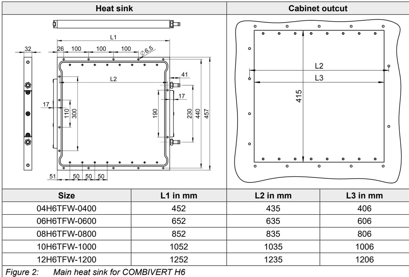
3.4.4 Dimensions and weights of modules with flat rear heat sink
