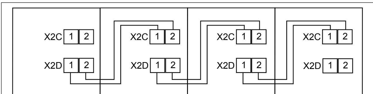
Figure 37: Wiring example error chain
