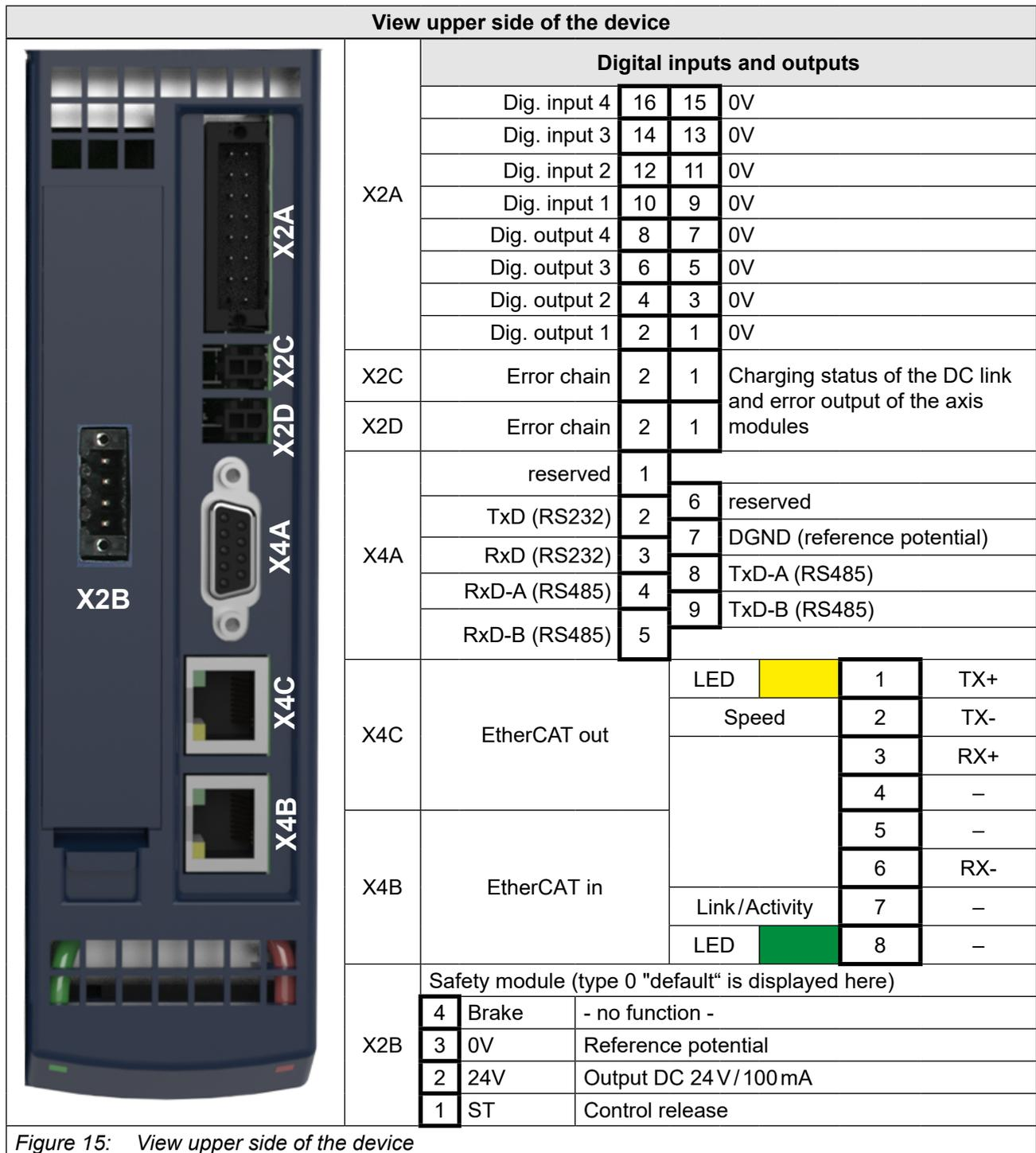
Figure 15: View upper side of the device
