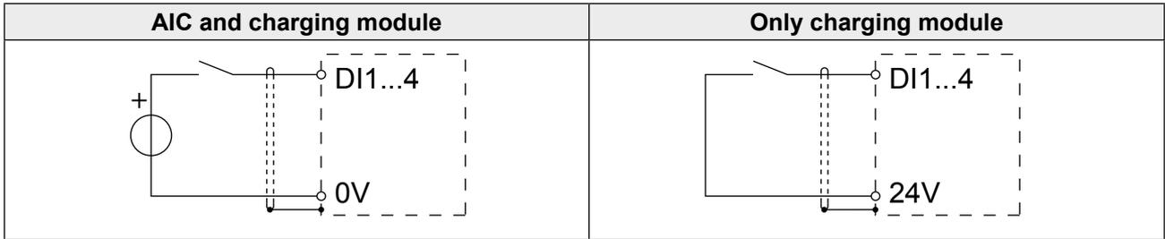
Figure 42: Connection of the digital inputs DI 1...DI 4
