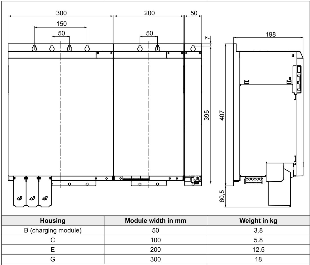
Figure 3: Dimensions and weights of the modules
