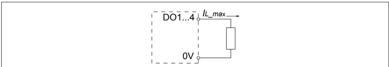
Figure 43: Connection of the digital outputs DO 1...DO 4
