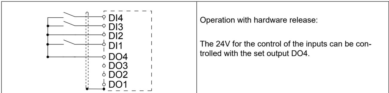
Figure 44: Example for the control of digital inputs and digital outputs
