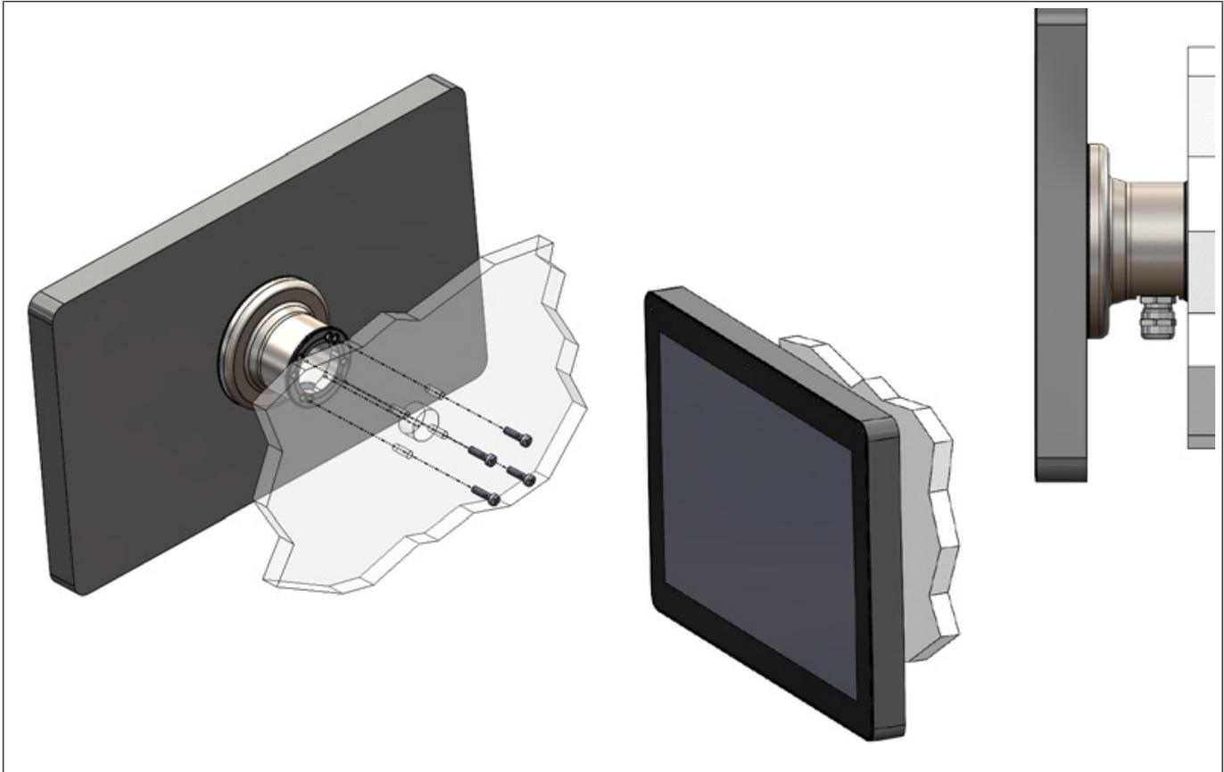
Fig. 2: Panel mounting C6 X1-M2
