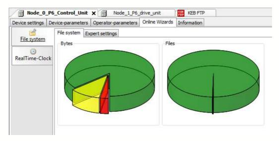
The yellow colour indicates that some files were deleted, but memory is not cleaned up (explained in step 4). To do it, click on "expert settings"-- double click on parameter *Fl07: flash function* – select *start cleanup* and click on "OK".
