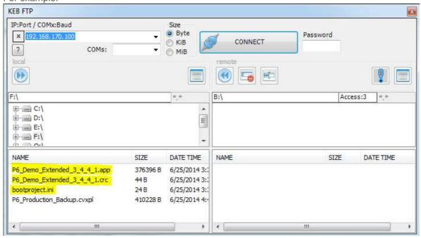
Enter P6 IP address and password. Then press "Connect", select drive "C" of the P6 control unit and transfer these 3 files to the P6 control unit, **one by one** (same behaviour as before with deleting files: it's not possible to send more than one file at the same time).
